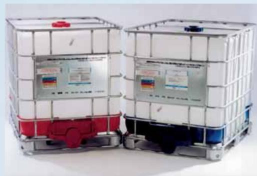
IBCs that contain Bayer Corporation polyurethane systems components are now color-coded to prevent accidental cross feeding in the field. IBCs that contain Bayer isocyanates (left) are equipped with red corner protectors, red fill port caps, red dust covers and red discharge valve protector plates. IBCs that contain Bayer polyols sport blue corner protectors, blue fill port caps, blue dust covers and blue discharge valve protector plates (right).
