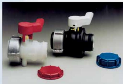
IBCs that contain Bayer isocyanates now feature a 2-inch male butterfly discharge valve with a Kam-Lok® quick disconnect fitting consistent with standards proposed by the European Isocyanate Producers Association (ISOPA), and a red valve cap (left). IBCs that contain Bayer polyols now have a standard 2-inch NPT threaded male ball-valve discharge outlet and a blue valve cap (right).
